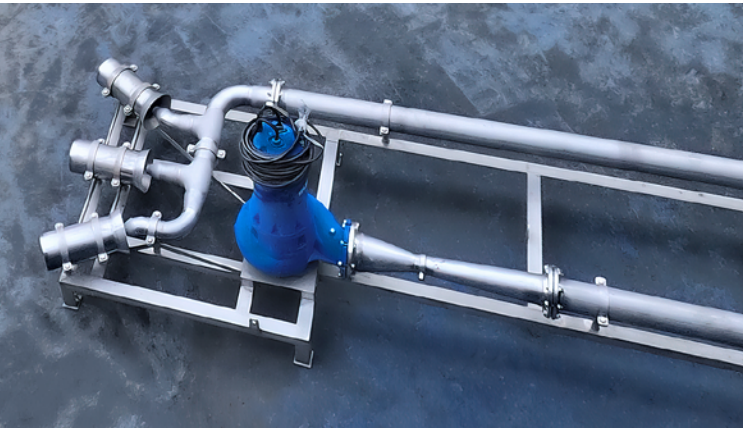
Messer BIOX injector for efficient dissolution of oxygen in water
