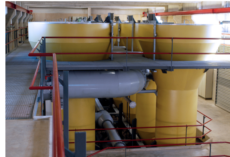
Fluidized bed reactor
