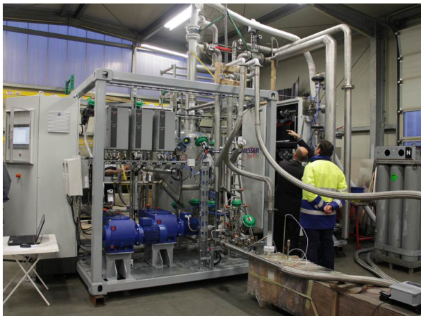
Fig. 3. Cooling unit, performance test at the manufacturer (Krytem GmbH, Willich).
