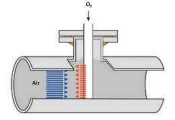
Oxygen mixer for combustion air enrichment
