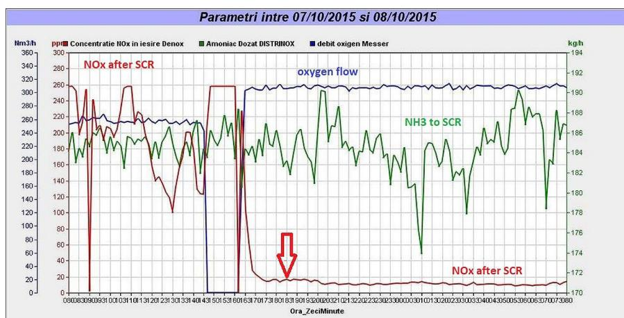
**Figure 6.** Plot of NO<sub>x</sub> values, ammonia consumption and oxygen flow. The red line indicates NO<sub>x</sub> emissions after DeNO<sub>x</sub> (limit value: 90 ppm). The green line indicates NH<sub>3</sub> consumption for DeNO<sub>x</sub>, which was kept at approximately 185 kg/hr. The blue line indicates oxygen consumption, which started at 260 Nm<sup>3</sup>/hr and increased to 310 Nm<sup>3</sup>/hr. NO<sub>x</sub> emission values decreased to 20 ppm.
