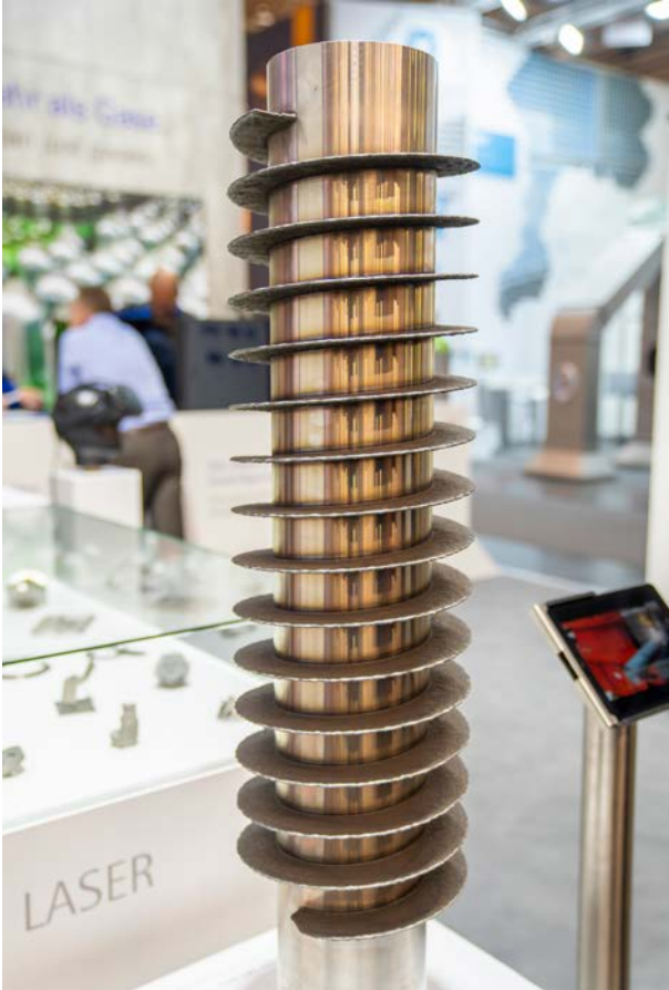
LMD-P printed screw conveyor
