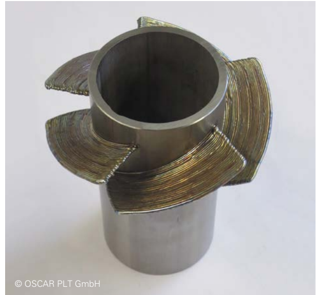
Coaxial laser metal deposition with wire
