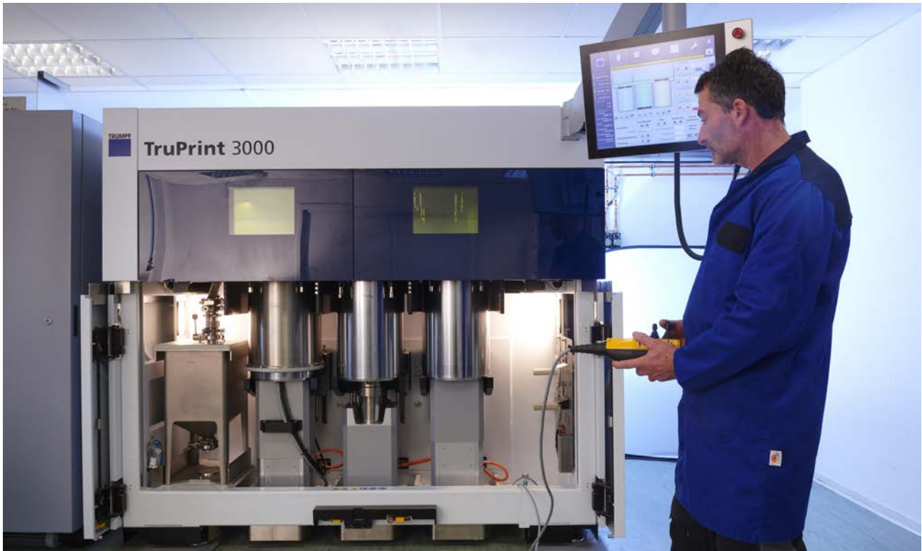
Powder change in a shielding gas atmosphere, carried out at ifw Jena
